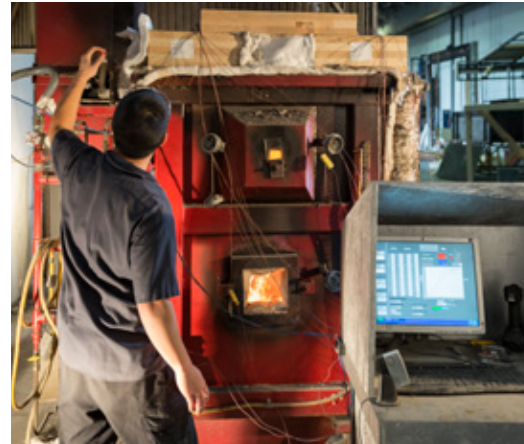
Fire testing of the CLT floor assembly
